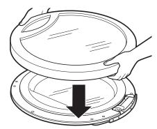
After reversing door, there will be a mismatch between the outer door and the inner door.
